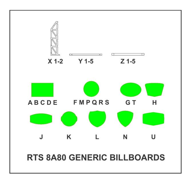
You will notice that this product is made up of a support structure and a specific billboard. The support structure is made up from two leg girders (**X 1-2**) and then five horizontal beams (**Z 1-5**) in front where the billboard will be attached too, as well as five bracing beams (**Y 1-5**) at the rear of the structure.
