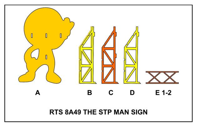
You will notice that this structure is made up of a man shaped billboard (A) that is supported by three legs (B), (C) and (D). NOTE: The man shaped billboard must be waving to the right as viewed from the front in order for the artwork supplied to fit. NOTE: The leg (C) is different from the other two and has two nubs and needs to go in the middle. The legs are braced at the rear by two braces (E 1-2).
