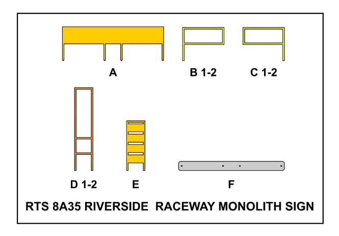
This can best be described as a "sandwich" design. The two outer layers is made up of parts (B 1-2), (C 1-2) and (D 1-2). The central layer is made up of parts (A) and (E). Part (A) will be glued into the foundation (F). Parts (B 1-2), (C 1-2) and (D 1-2) will be glued to part (A). Part (E) will fit on top of part (A) and between parts (D 1-2).
