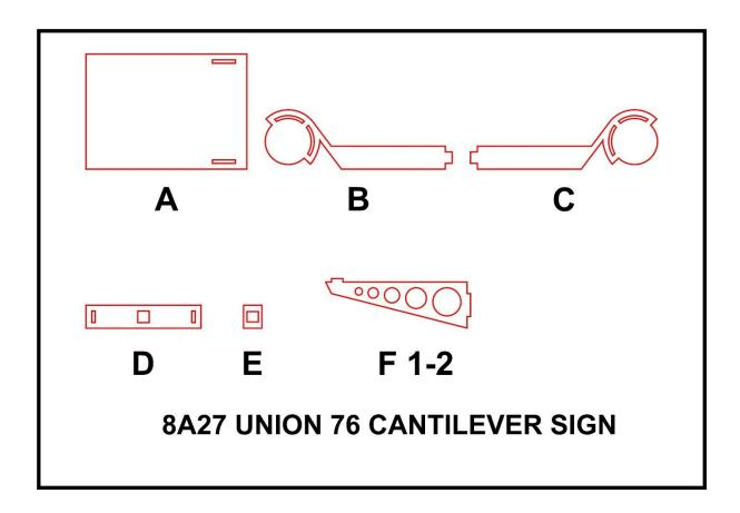
You will notice that this structure is made up of two legs (**F 1-2**) that supports a small cross beam (**D**) at the top. The bottom of the legs fits into the base plate (**A**). The two cantilever beams (**B & C**) are fixed to the cross beam with a clip (**E**) to keep them in place.
