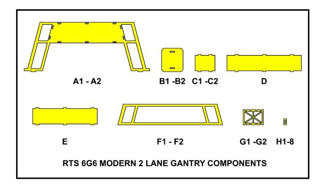
The gantry has two girder sides (A1 - A2) that fits into two foundations (B1 - B2). There are two vertical box sides (C1 - C2), a box floor (D) and a box roof (E). There are two frames (F1 - F2) that fits onto the outsides of the two girder sides (A1 - A2). Lastly there are two leg braces (G1 - G2) that must be fixed between the leg portions of the two sides with "shoes" (H 1-8).
