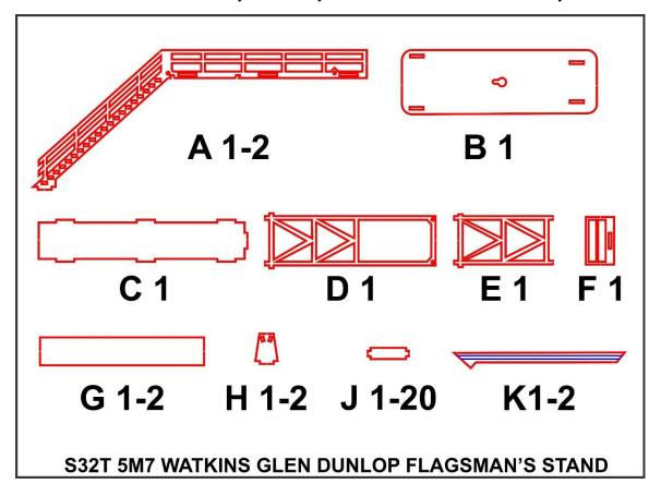
You will notice that the main structure consists of two sides (A1-2), a foundation (base plate) (B1), a floor (C1), two support legs (D1) and (E1), as well as some steps (J 1-20). Please identifies the two slots on the underside of the horizontal part of the walkway. This is where the two supporting legs will fit in later.
