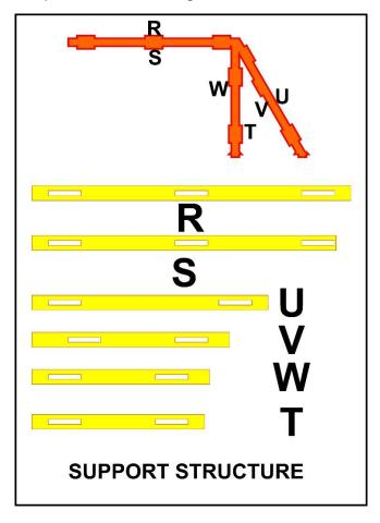
Have a look at the diagram with all the components. It clearly indicates where each flange fits to the web. All that needs to be done is to glue the different flanges (**R**, **S**, **T**, **U**, **V** and **W**) to the web (**P**). Allow the glue to set fully before the completed I-beam is glued to the base (**Q**).
