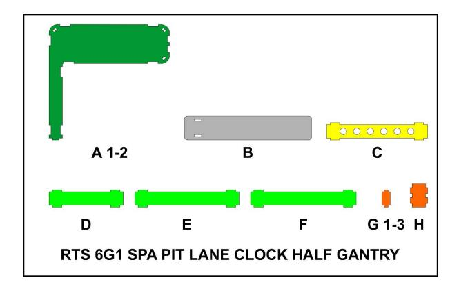
The structure has a base plate (**B**) to which the two main sides (**A1-2**) of the gantry will be fixed. The two sides of the column part of the gantry are pieces (**D**) and (**E**). The top of the gantry is enclosed by piece (**F**). The three corners are closed by (**G 1-3**) and the short side by piece (**H**). The underside of the gantry is closed off by piece (**C**), which have holes so that a light can be fitted inside the box of the gantry.
