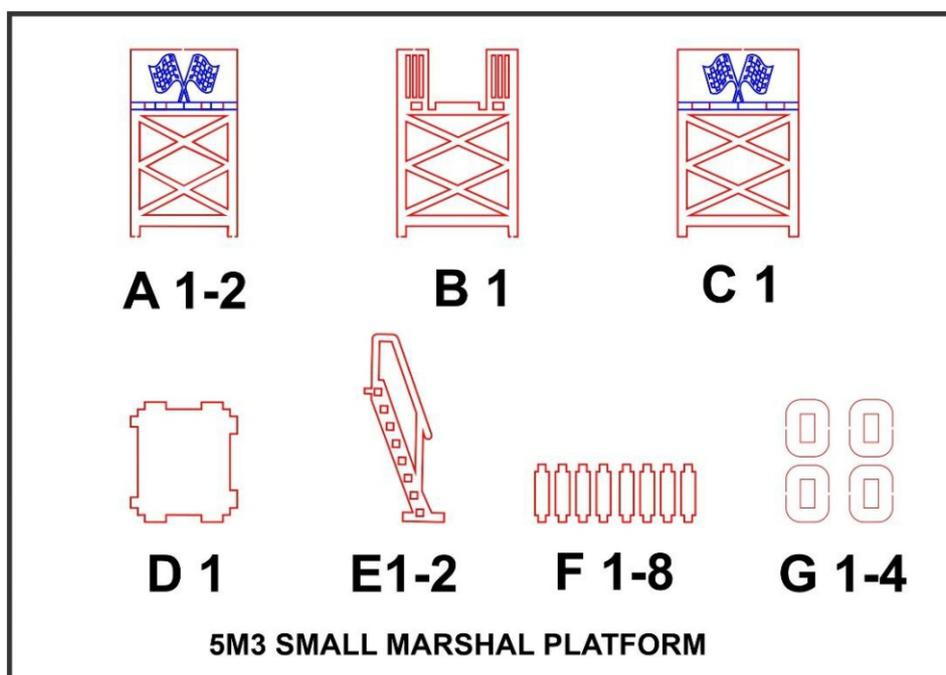
You will notice that the small structure consists of four sides (**A1-2**), (**B1**) and (**C 1**) and a floor (**D 1**). There are also the two sides of the ladder (**E 1-2**) and some steps (**F 1-8**). Lastly, you will notice the four small foundations (**G1-4**) for the legs.
