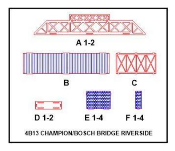
You will notice that the main bridge structure consists of two sides (A1-2) and the floor piece (B) as well as a top brace (C). The original bridge was situated between two earth embankments but we thought that we are going to include some buttress that can be used in the absence of embankments on your track. The buttresses each consists of a base plate (D), two long walls (E) and two short walls (F).
