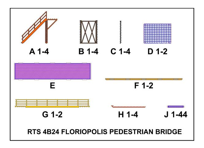
The bridge structure consists of two staircases and a super structure (deck). Each staircase is made up of two sides (A 1-4), two leg braces, (B 1-4), two column sides (C 1-4), a foundation (D 1-2), two step-supports (H 1-4) and 22 threads (J 1-44).
