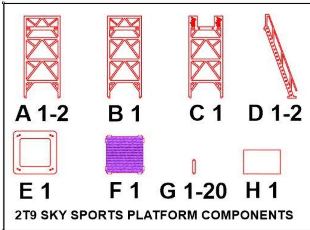
The structure has a base plate (**E 1**) and the four legs (**A 1-2**), (**B 1**) and (**C 1**) fits into this base plate. The one leg (**C 1**) has some engraving that must face outwards if you want it visible. The floor (**F 1**) fits into the four legs. Ensure that the engraving faces upwards if you want it visible. There is an advertising board (**H 1**) that will be glued to the front leg. Lastly there are the two sides of the ladder (**D 1-2**) and the individual steps (**G 1-20**)
