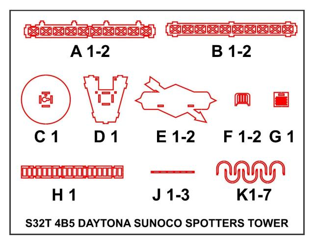
The structure has a base plate (**C**) to which the four sides of the column (**A1-2**) and (**B1-2**) will be fixed. You will notice that there is a round opening in the base plate if you want to feed an electrical cable to a light in the structure. There is also a keyhole for attaching the tower to your race track.
