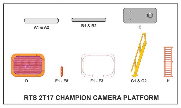
Now have a look at the next diagram where all the laser cut parts are showed and numbered from **A** to **H** and try to identify which is which and where they fit in.
