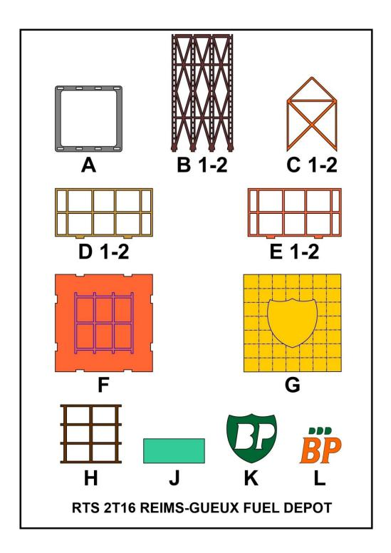
The tower structure stands on two sets of legs (**B 1-2**) that fits into a ring-beam foundation (**A**). This is not visible above ground on the photos above but helps to ensure a sturdy assembly. Between the two sets of legs, on each end is some bracing (**C 1-2**), that can be seen in the last photo of the restored structure above.
