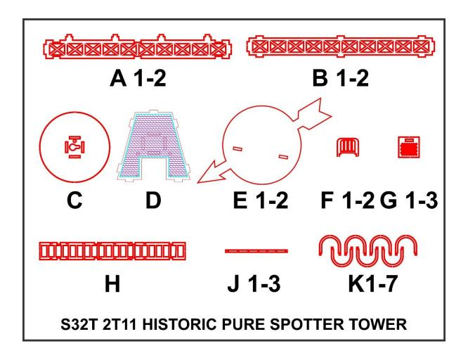
The structure has a base plate (**C**) to which the four sides (**A1-2**) and (**B1-2**) of the column will be fixed. You will notice that there is a round opening in the base plate if you want to feed an electrical cable to a light in the structure. There is also a keyhole for attaching the tower to your race track.
