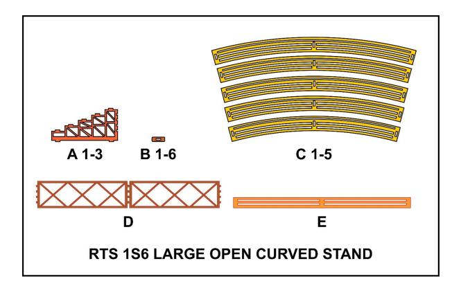
You will notice that this stand is made up of five seats (**C 1-5**) that are supported by three girder legs (**A 1-3**). Each leg has two small foundations (**B 1-6**). On top of the highest seat is a back rest (**E**) and access to the structure from the back is restricted by a trellis fence (**D**).
