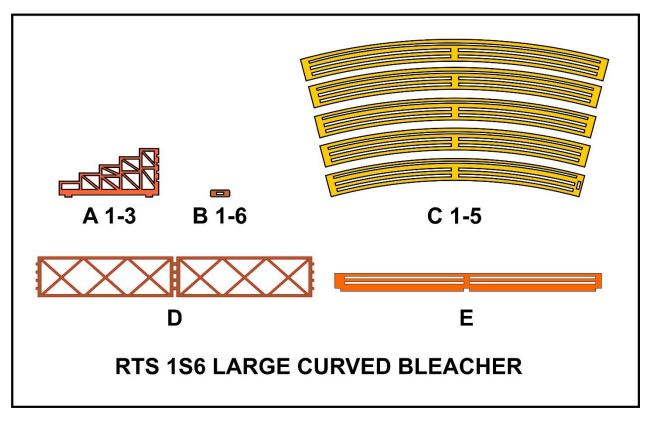
You will notice that this bleacher is made up of five seats (**C 1-5**) that are supported by three girder legs (**A 1-3**). Each leg has two small foundations (**B 1-6**). On top of the highest seat is a back rest (**E**) and access to the structure from the back is restricted by a trellis fence (**D**).
