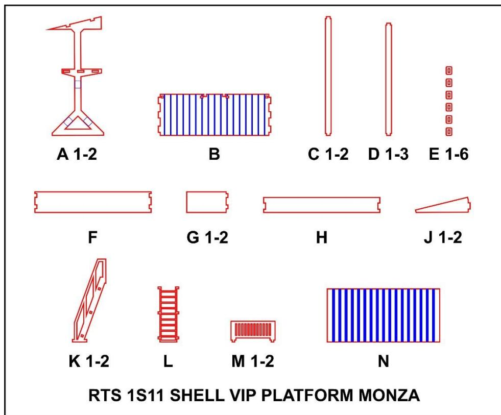
The structure consists of two legs (**A 1-2**) that support the floor (**B**). There are two roof beams (**C 1-2**) that span from one leg to the other. There are a further three beams (**D 1-3**) that connects the two legs below the level of the floor. These beams are attached to the legs with the use of "shoes" (**E 1-6**). (They are slightly shorter than the roof beams).
