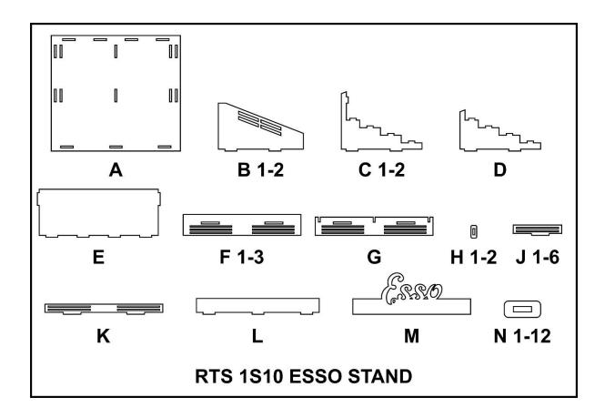
The side walls (**B 1-2**), the rear wall (**E**), the low front wall (**L**), as well as the supports (**C 1-2**) and (**D**) fits into the floor (**A**). Support (**D**) is the centre support.
