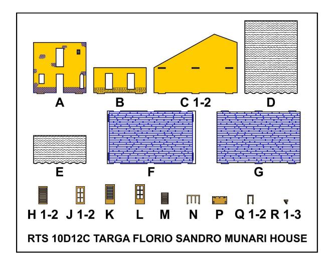
The front wall (A), the rear wall (B) and the side walls (C 1-2) fit into the foundation floor (F). There are two parts for the roof (D) and (E) and a first floor (G). The louvres (H 1-2) and window frames (J 1-2) will be used for the rear wall. The louvre door (K), the door (L) and the louvre (M) will be used for the front wall. There is also a balcony that is made up of parts (N), (P), (Q 1-2) and (R 1-3) that will form part of the front wall.
