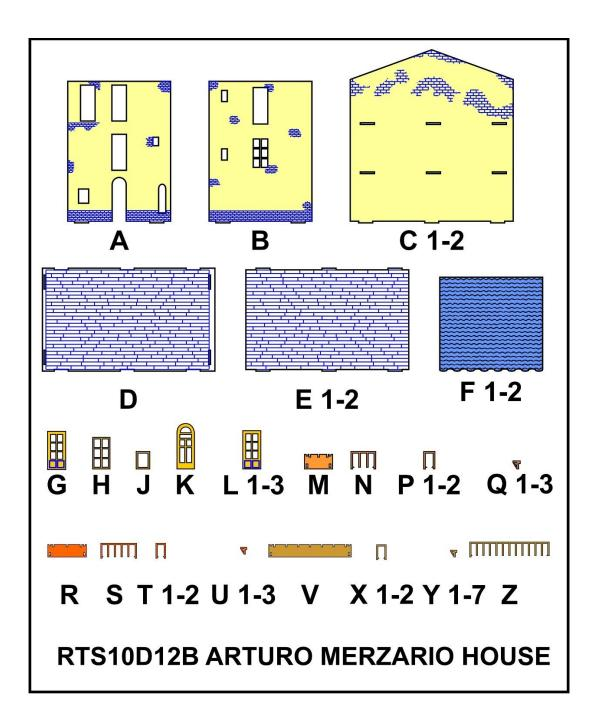
The front wall (A), the rear wall (B) and the side walls (C 1-2) fit into the foundation floor (D). There are two parts for the roof (F 1-2) and a first and second floor (E 1-2). The door (G), the window frame (H), as well as the balcony (R, S, T 1-2 & U 1-3) will be used for the rear wall.
